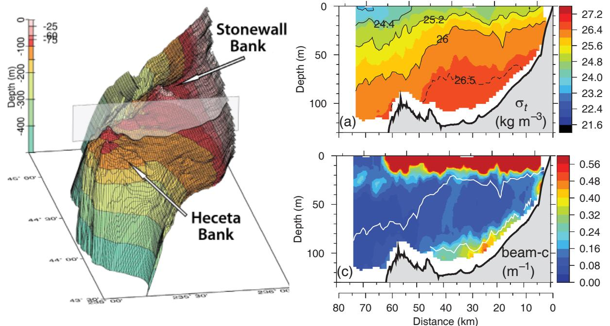
Cross-shelf vertical sections of density and light attenuation from over Heceta Bank, Oregon, measured with the towed, undulating vehicle SeaSoar. (From Barth et al. 2005.)
